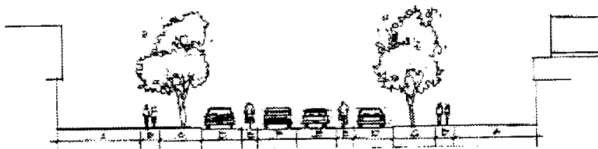
Cross-section of a typical Main Street with the recommended dimensions of each component: A) building setback from street right-of-way; B) sidewalk;
